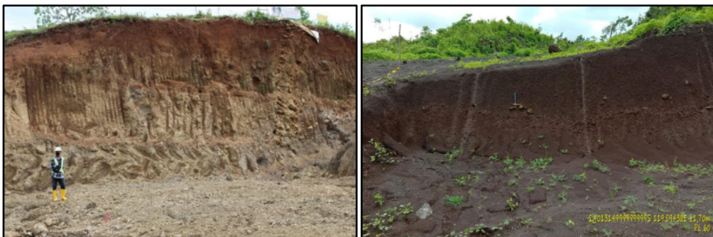
Figure 7. Residual soil found in Pamukkulu dam area, South Sulawesi, Indonesia
