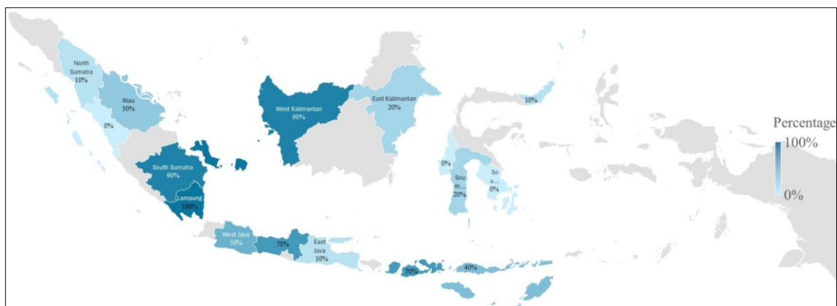
Figure 9. Distribution of percentage pile with defects
