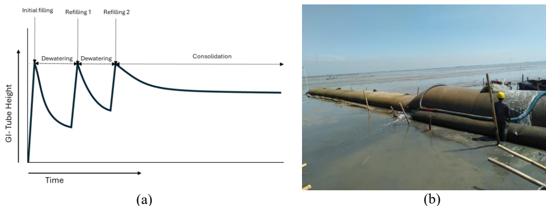
Figure 8. (a) Typical cycles of GI-Tube filling process, (b) GI-Tube filling process
