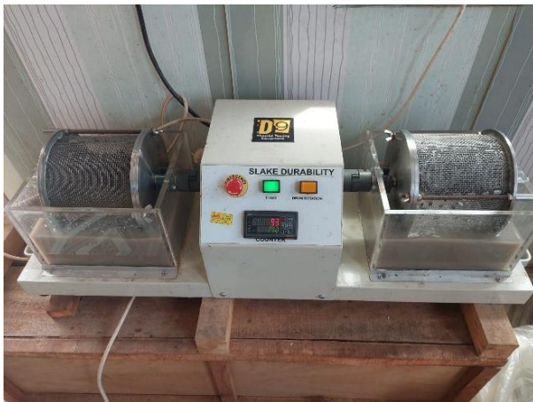
Figure 12. Slake durability tool
