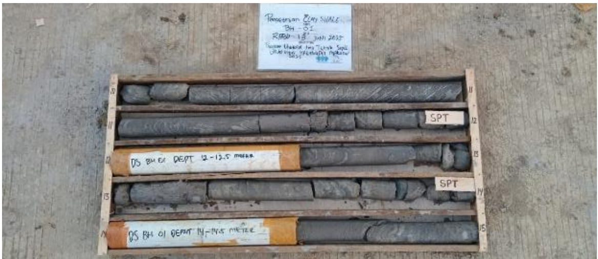
Figure 13. BH. 01 & 02 borelogs, and enlarged photographs of BH-01 coreboxes (0 to 5 m & 10 to 15 m)
