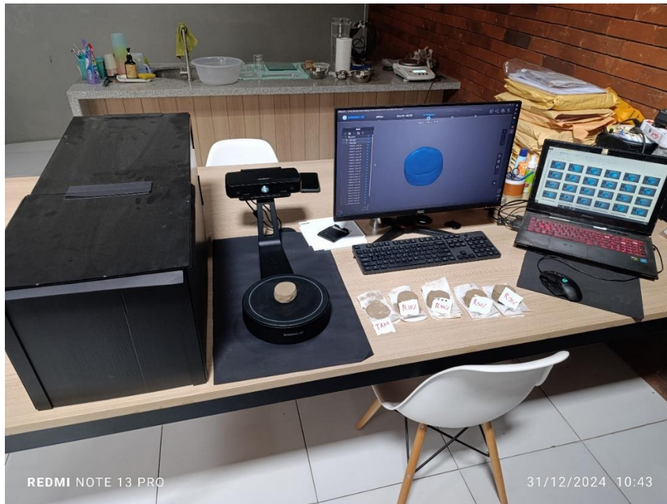
Figure 7 The 3 - D Scanner for measuring volume change
